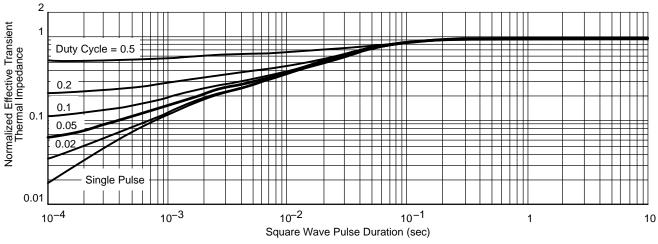
Figure 12. Normalized Thermal Transient Impedance, Junction-to-Foot
