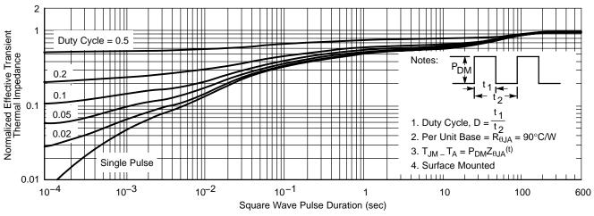
Figure 11. Normalized Thermal Transient Impedance, Junction-to-Ambient
