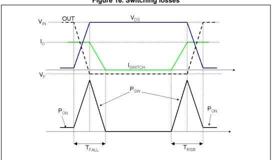
Figure 16. Switching losses
