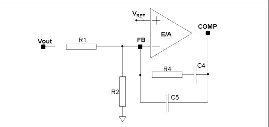
Figure 13. Type II compensation network
