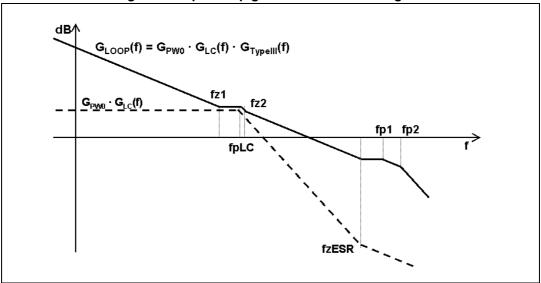
Figure 11. Open loop gain: module Bode diagram
