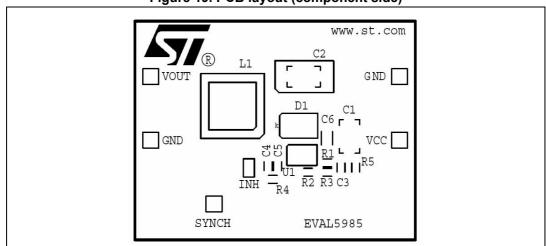
Figure 19. PCB layout (component side)
