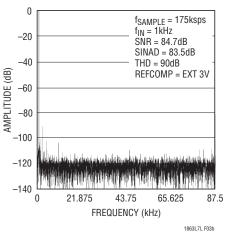
Figure 3b. LTC1867L Nonaveraged 4096 Point FFT Plot with 3V Supply
