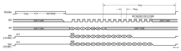
Figure 6. Example 1, CS/CONV Starts a Conversion and Remains HIGH Until Next Data Transfer. With CS/CONV Remaining HIGH After the Conversion, Automatic Nap Modes Provides Power Reduction at Reduced Sample Rate
