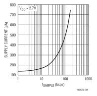
Figure 5. Supply Current vs f<sub>SAMPLE</sub>
