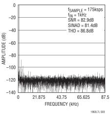
Figure 3a. LTC1867L Nonaveraged 4096 Point FFT Plot with 2.7V Supply
