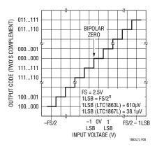
Figure 8. LTC1863L/LTC1867L Bipolar Transfer Characteristics (Two's Complement)
