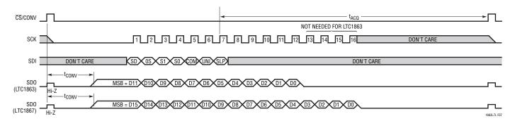
Figure 7. Example 2,  $\overline{\text{CS}}$ /CONV Starts a Conversion With Short Active HIGH Pulse. With  $\overline{\text{CS}}$ /CONV Returning LOW Before the Conversion, the ADC Remains Powered Up
