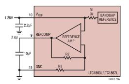
Figure 4a. LTC1867L Reference Circuit
