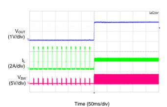
Load Transient (I<sub>OUT</sub>=0.1A to 2A)
