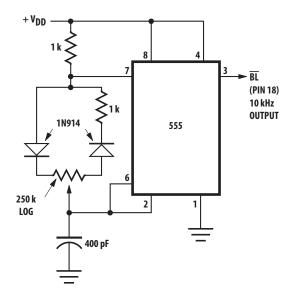
Figure 3 shows a circuit designed to dim the display from 98% to 2% by pulse width modulating the BL input. A logarithmic or a linear potentiometer may be used to adjust the display intensity. However, a logarithmic potentiometer matches the response of the human eye and therefore provides better resolution at low intensities. The circuit frequency should be designed to operate at 10 kHz or higher. Lower frequencies may cause the display to flicker.
