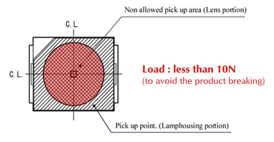
Please adjust the load, the pick up point, the nozzle diameter, etc. before mounting because the over load can cause the breakage of the lamp housing.
