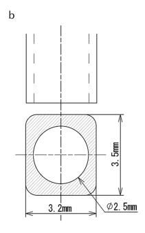
Nozzle with chamfering is recommended
