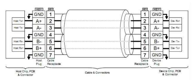
Figure 3-2 SATA Cable / Connector Connection Diagram
