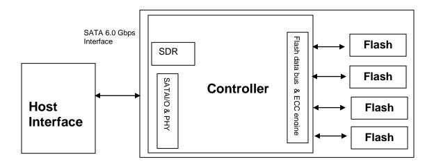
Figure 2-1 Apacer CFast Block Diagram
