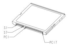
Figure 3-1 Pin Assignment
