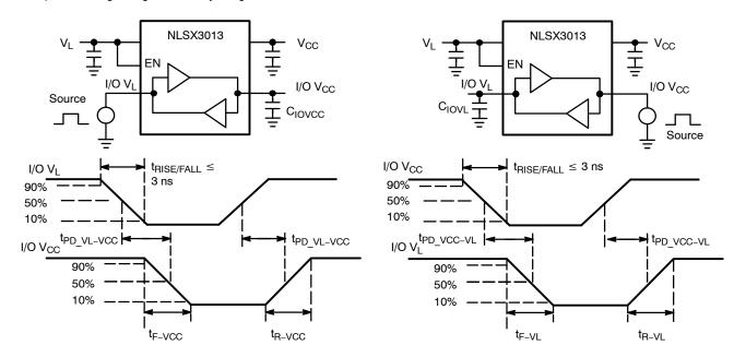
Figure 4. Driving I/O V<sub>L</sub> Test Circuit and Timing
