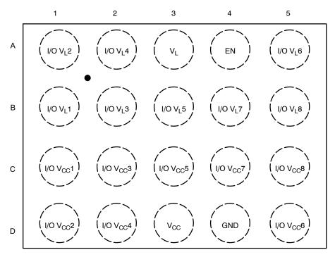
Figure 3. 20 Flip-Chip (2.54 mm x 2.03 mm) (Top View)
