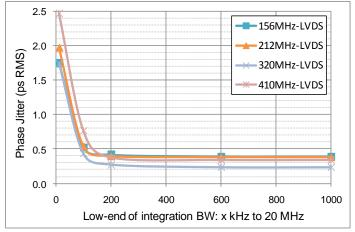
LVDS Phase jitter (integrated phase noise)
