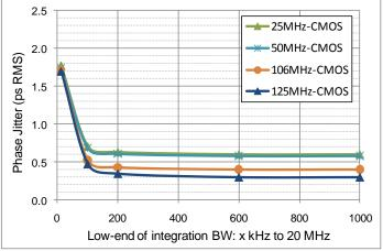
CMOS Phase jitter (integrated phase noise)
