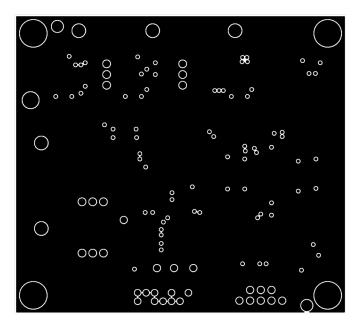
Figure 18. Layer 2 GND Plane
