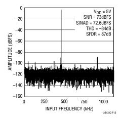
Figure 13. 16k Point FFT of the LTC2313-12 at  $f_{IN} = 497kHz$
