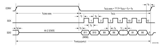
Figure 5. LTC2313-12 Serial Interface Timing Diagram (SCK Low During t<sub>CONV</sub>)
