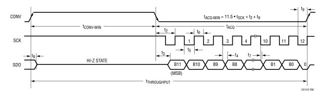
Figure 6. LTC2313-12 Serial Interface Timing Diagram (SCK High During t<sub>CONV</sub>)
