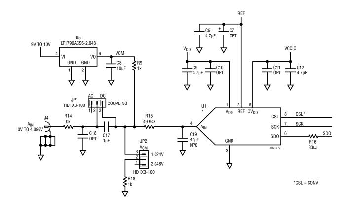
Figure 21. Partial 1563 Demo Board Schematic
