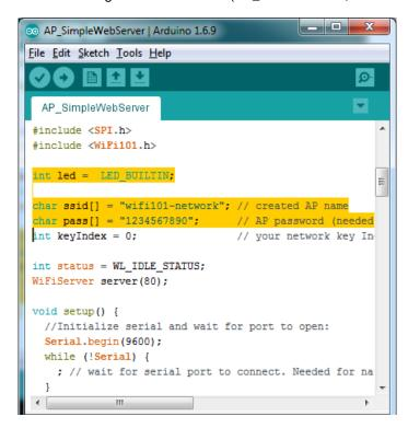
Upload and open up the serial console to start the AP
