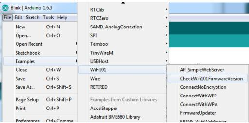
Note that to use the official Arduino WiFi101 Library, we must configure it to use the pins specific to the ATWINC1500 Feather. With each example sketch, you'll need to add WiFi.setPins(8,7,4,2); to the top of the setup function!
