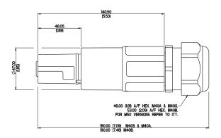
Line Drain is the connector with a female contact which is not normally the live part, however they are fitted with a spring loaded plastic cap that prevents accidental finger touching of the contact, and the connector meets IP2X requirements. Contacts are available to suit cable conductors from 25mm2 to 300mm2.
