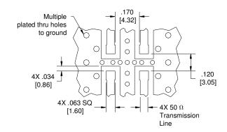
Dimensions are in Inches [Millimeters] 1P520S Mounting Footprint
