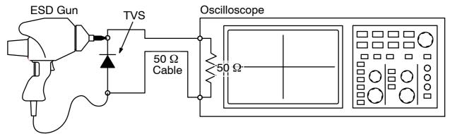
Figure 4. Diagram of ESD Test Setup
