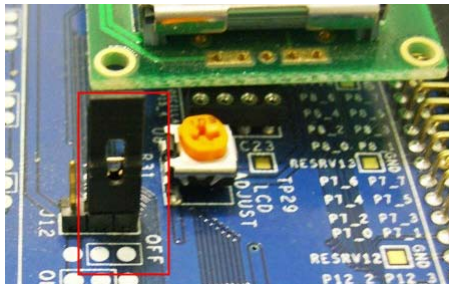
Figure 4-6. J12 Jumper in Off Position
