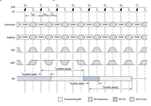
Figure 83: ODT Turn-Off Timings When Entering Power-Down Mode
