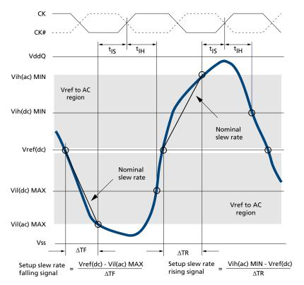
Figure 23: Tangent Line for <sup>t</sup>IS
