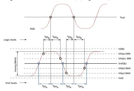
Figure 33: AC Input Test Signal Waveform (Differential)
