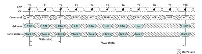
Note: 1. DDR2-533 (-37E, x4 or x8), <sup>t</sup>CK = 3.75ns, BL = 4, AL = 3, CL = 4, <sup>t</sup>RRD (MIN) = 7.5ns, <sup>t</sup>FAW (MIN) = 37.5ns.
