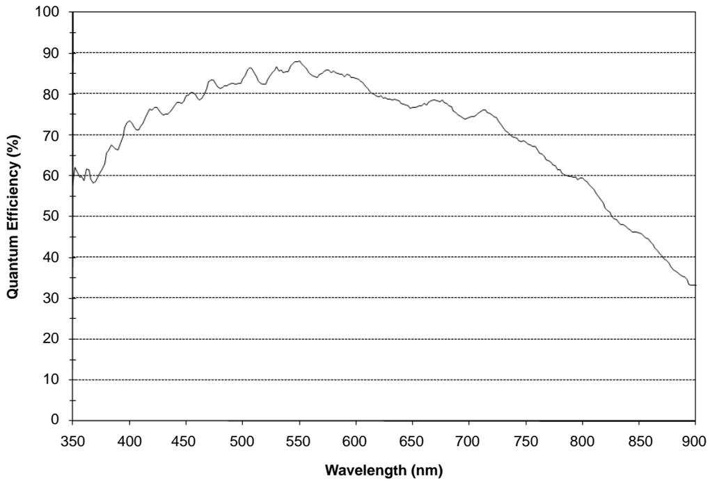
Figure 9. KLI-2104 Quantum Efficiency – Even/Odd Monochrome Channels
