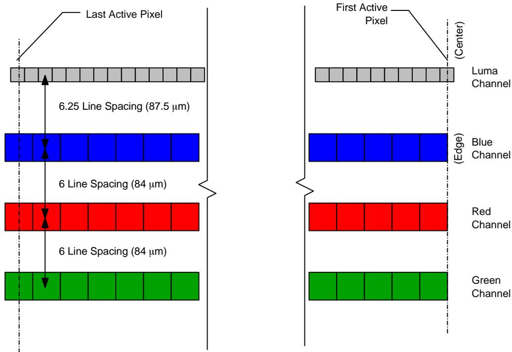
Figure 4. Active Pixel and Channel Alignment – KLI-2104
