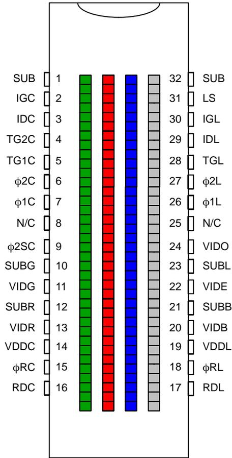
Figure 5. Pinout Diagram
