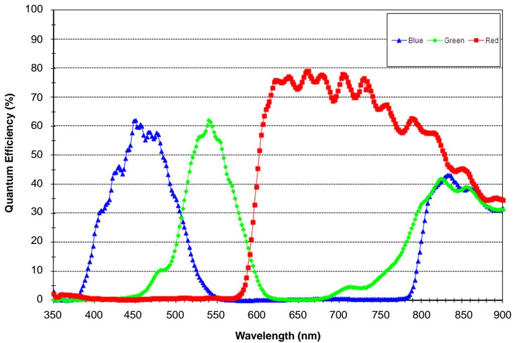
Figure 10. KLI-2104 Quantum Efficiency – Color Channels
