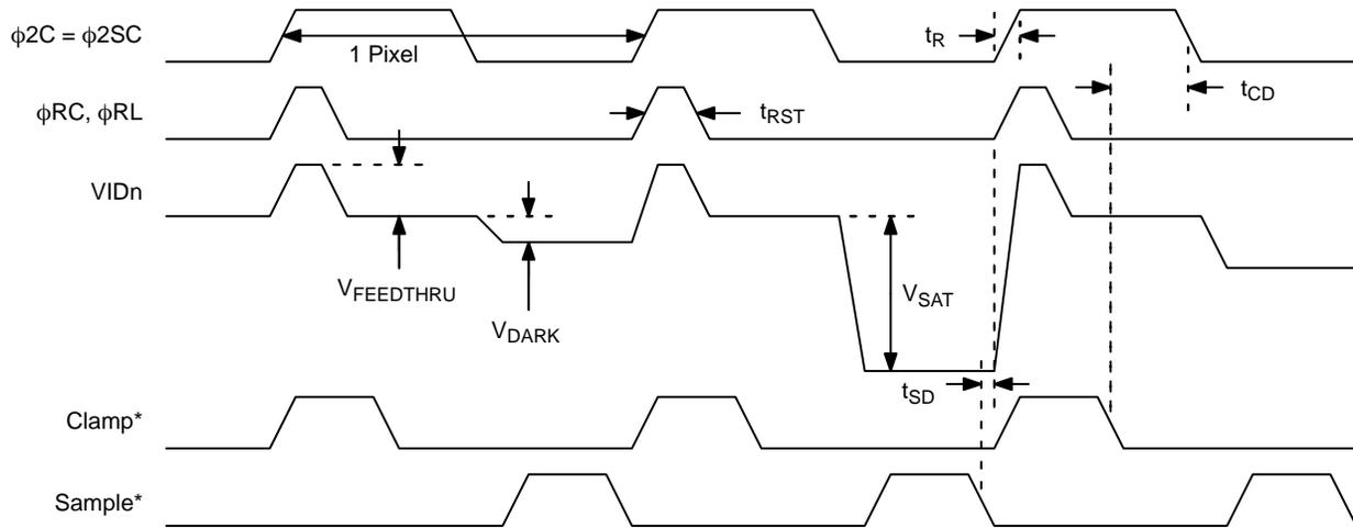
**Output Timing – 2-Pixel Summing Mode**
