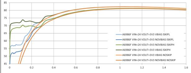
Figure 62. Efficiency curves:  $V_{IN}$  = 24 V -  $V_{OUT}$  = 3.3 V - fsw = 500 kHz (log scale)
