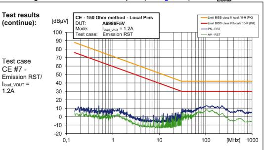
Figure 70. CE 150R at RST test point (see Figure 65) at 80% ILOAD
