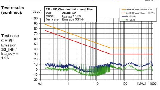
Figure 72. CE 150R at SS/INH test point (see Figure 65 on page 70) at 80% ILOAD
