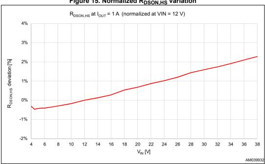
Figure 15. Normalized R<sub>DSON.HS</sub> variation
