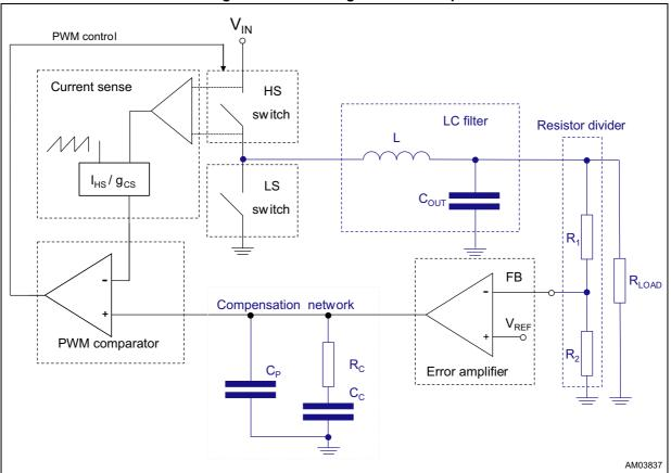
Figure 36. Block diagram of the loop
