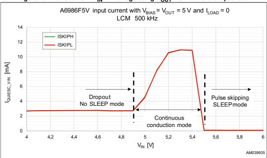
Figure 29. Current from  $V_{IN}$  while regulating  $V_{OUT}$  = 5 V at zero output load
