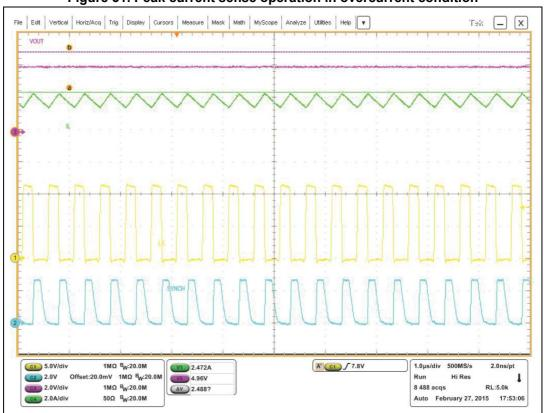
Figure 31. Peak current sense operation in overcurrent condition
