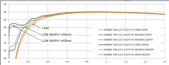
Figure 18. Light-load efficiency comparison at different I<sub>SKIP</sub> - linear scale
