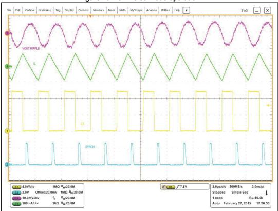
Figure 16. Low noise mode operation
