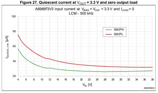
When  $V_{IN}$  is adequately higher than  $V_{OUT}$  (see *Figure 27*) the device works in the bursts mode operation, minimizing the power consumption over the entire input voltage (see *Section 5.8.2: Low consumption mode (LCM)*).
