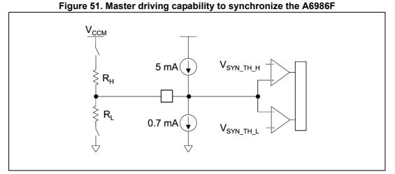
As anticipated above, in SLAVE mode the internal oscillator operates at 250 kHz typ. but the slope compensation is dimensioned accordingly with FSW resistors so, even if the A6986F supports synchronization over the 275 kHz - 1.4 MHz frequency range, it is important to limit the switching operation around a working point close to the selected frequency (FSW resistor).
