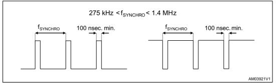
Figure 48. Synchronization pulse definition
