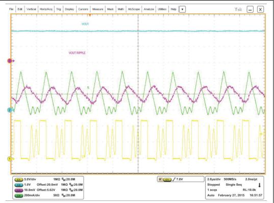
Figure 24. LCM operation over loading condition (part 3 - DCM)
