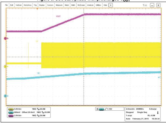
Figure 6. Soft-start phase with precharged COUT
