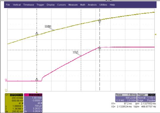
Figure 8. External soft-start network V<sub>STEP</sub> driven
