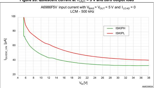
Figure 28. Quiescent current at  $V_{OUT}$  = 5 V and zero output load
