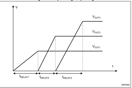
Figure 12. Output voltage sequencing
