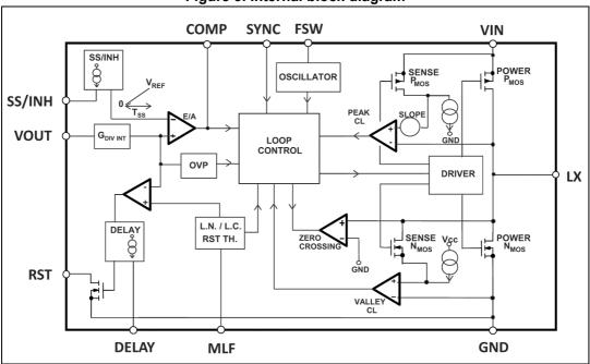
Figure 3. Internal block diagram
