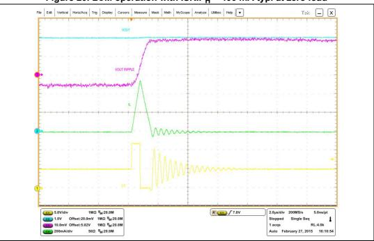
Figure 20. LCM operation with  $ISKIP_{H}$  = 400 mA typ. at zero load
