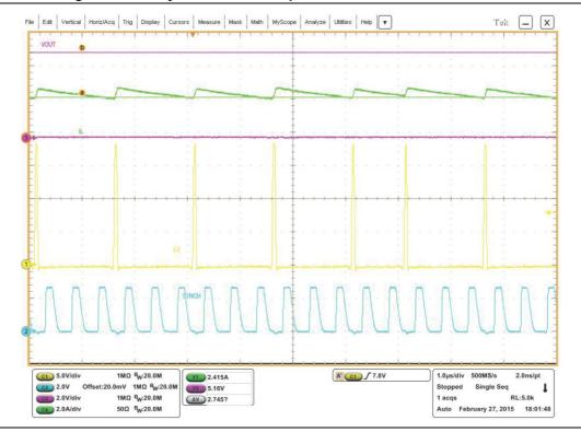
Figure 30. Valley current sense operation in overcurrent condition
