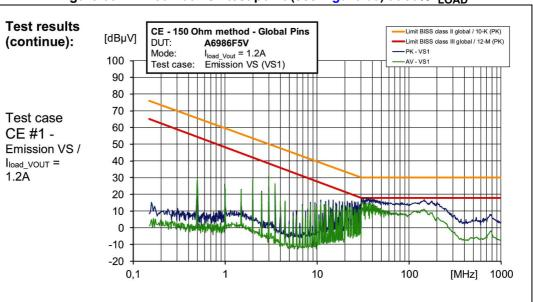
Figure 66. CE 150R at VS1 test point (see Figure 65) at 80% ILOAD
