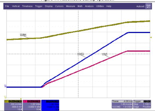
Figure 11. Ratiometric startup operation
