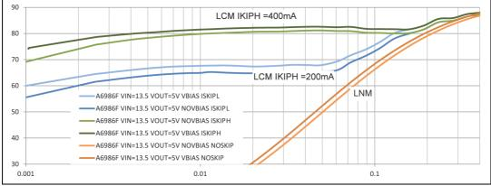
*Figure 20* and *Figure 21* show the LCM operation at the different ISKIP level. *Figure 20* shows the ISKIP<sub>H</sub> = 400 mA typ. and so 20 mV output voltage ripple. *Figure 21* shows the ISKIP<sub>L</sub> = 200 mA typ. and so 10 mV output voltage ripple.
