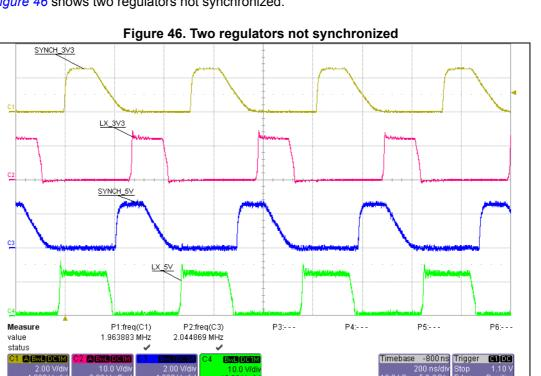
Figure 46 shows two regulators not synchronized.
