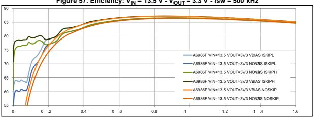
Figure 57. Efficiency:  $V_{IN}$  = 13.5 V -  $V_{OUT}$  = 3.3 V - fsw = 500 kHz
