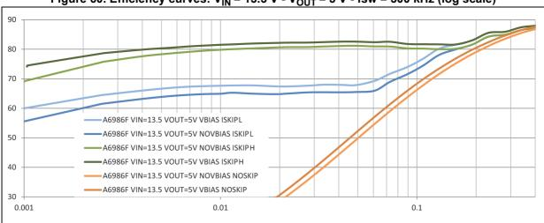
Figure 60. Efficiency curves:  $V_{IN}$  = 13.5 V -  $V_{OUT}$  = 5 V - fsw = 500 kHz (log scale)
