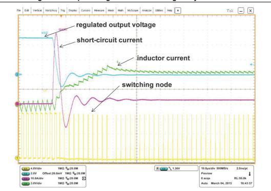
Figure 32. Output voltage oscillations during heavy short-circuit
