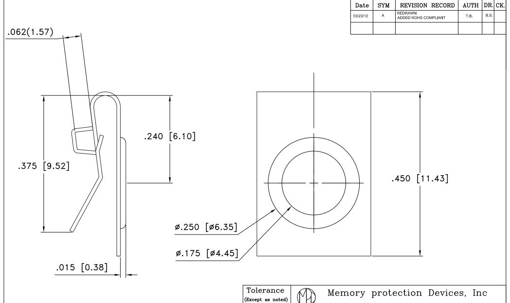
MATERIAL: 0.010" SPRING TEMPER STAINLESS STEEL, NICKEL PLATED ROHS COMPLIANT
