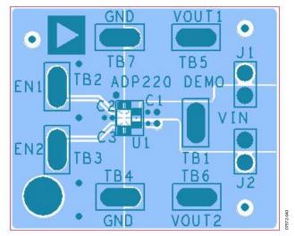
Figure 40. Example of PCB Layout, Top Side
