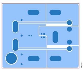
Figure 41. Example of PCB Layout, Bottom Side
