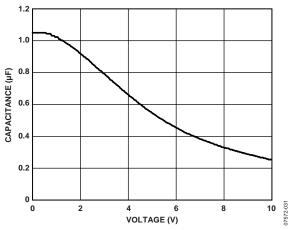
Figure 31. Capacitance vs. Voltage Bias Characteristic
