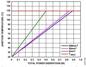
Figure 35. Junction Temperature vs. Total Power Dissipation,  $T_A = 25^{\circ}C$
