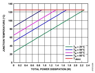
Figure 39. Junction Temperature vs. Total Power Dissipation and Board Temperature
