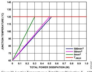
Figure 37. Junction Temperature vs. Total Power Dissipation,  $T_A = 65^{\circ}C$
