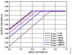
Figure 15. Output Voltage vs. Input Voltage (In Dropout)
