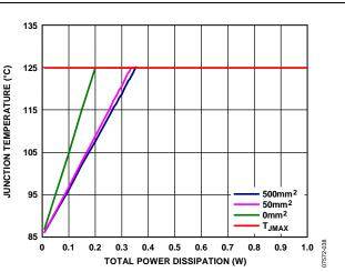
Figure 38. Junction Temperature vs. Total Power Dissipation,  $T_A = 85^{\circ}C$
