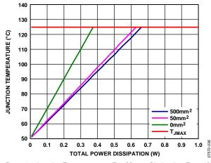
Figure 36. Junction Temperature vs. Total Power Dissipation,  $T_A = 50^{\circ}C$
