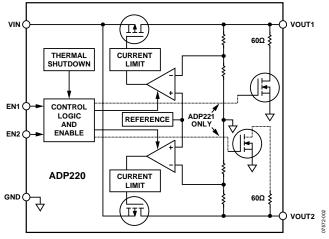
Figure 2. Block Diagram of the ADP220/ADP221
