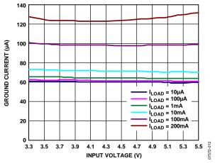
Figure 12. Ground Current vs. Input Voltage, Both Outputs Loaded
