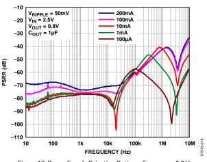
Figure 19. Power Supply Rejection Ratio vs. Frequency, 0.8 V
