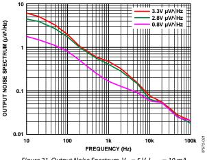
Figure 21. Output Noise Spectrum,  $V_{IN} = 5 V$ ,  $I_{LOAD} = 10 mA$
