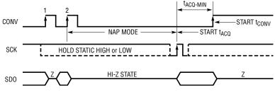
Figure 8. LTC2313-14 Entering/Exiting Nap Mode
