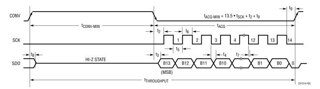
Figure 5. LTC2313-14 Serial Interface Timing Diagram (SCK Low During t<sub>CONV</sub>)
