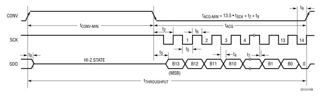
Figure 6. LTC2313-14 Serial Interface Timing Diagram (SCK High During t<sub>CONV</sub>)
