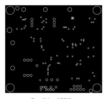
Figure 18. Layer 2 GND Plane
