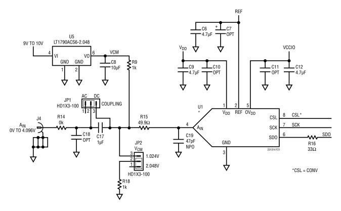
Figure 21. Partial 1563 Demo Board Schematic
