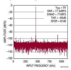
Figure 13. 16k Point FFT of the LTC2313-14 at f<sub>IN</sub> = 497kHz
