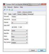
The SNAP Link EasySet software applet is an easy-to-use configuration tool that streamlines the setup and configuration of SNAP Link wireless adapters. SNAP Link EasySet provides visual indicators and easy-to-change configuration parameters such as baud rate, channel and network ID, data bits, parity, stop bits, flow control and more. SNAP Link EasySet is a visually intuitive tool for defining and configuring the SNAP Link products.
