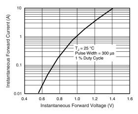
Figure 3. Typical Instantaneous Forward Characteristics
