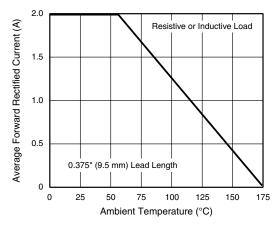
Figure 1. Forward Current Derating Curve
