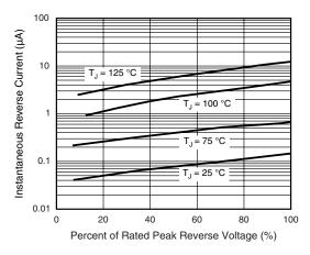
Figure 4. Typical Reverse Characteristics
