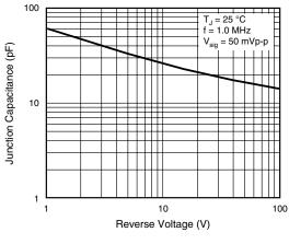
Figure 5. Typical Junction Capacitance
