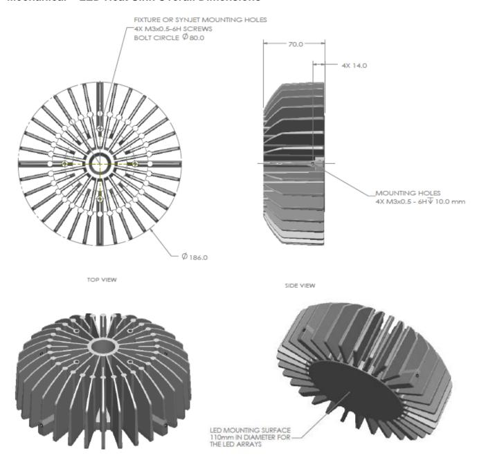
All dimensions are nominal and in mm unless otherwise stated. See product drawings for LED Mounting Surface Hole Patterns.
