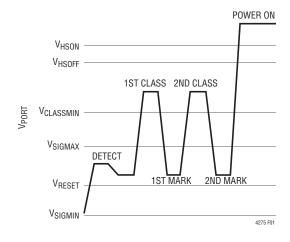
Figure 2. Type 2 Detect/Class Signaling Waveform
