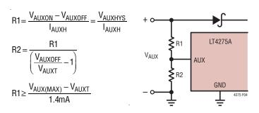
Figure 4. AUX Threshold and Hysteresis Calculation
