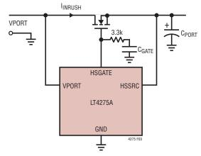
Figure 3. Programming I<sub>INBUSH</sub>
