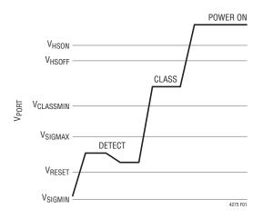
Figure 1. Type 1 Detect/Class Signaling Waveform
