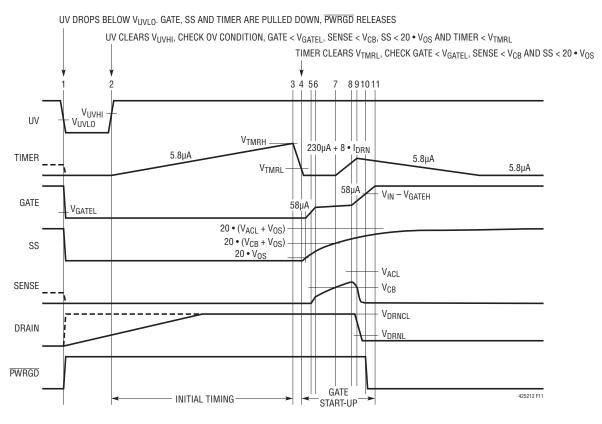
Figure 11. Undervoltage Timing (All Waveforms Are Referenced to  $V_{EE}$ )
