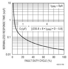
Figure 5. Circuit-Breaker Response Time
