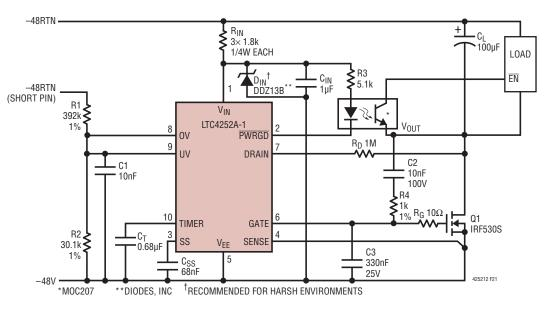
Figure 21. Inrush Control Without a Sense Resistor Application
