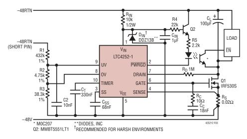
Figure 3. – 48V/2.5A Application with Different Input Operating Range
