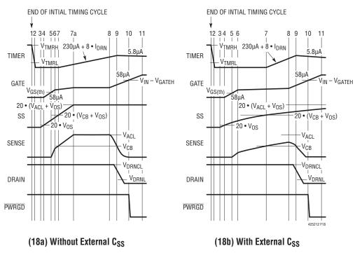
Figure 18. Soft-Start Timing (All Waveforms Are Referenced to V<sub>EE</sub>)
