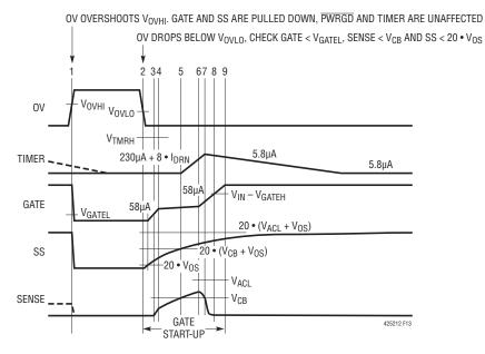
Figure 13. Overvoltage Timing (All Waveforms Are Referenced to  $V_{EE}$ )
