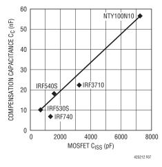
Figure 7. Recommended Compensation Capacitor  $C_C$  vs MOSFET  $C_{ISS}$
