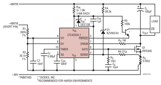
Figure 19. Power Limit Circuit Breaking Application
