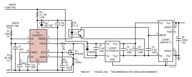
Figure 23. Typical Application Using a Filter Module
