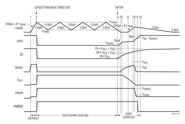
Figure 16. Shutdown Cooling Timing Behavior of LTC4252-2 (All Waveforms Are Referenced to V<sub>EE</sub>)
