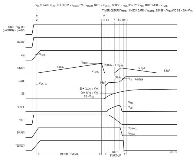
Figure 9. System Power-Up Timing (All Waveforms Are Referenced to V<sub>EE</sub>)
