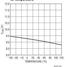
**Analog Current Limit Voltage V<sub>ACL</sub> vs** Temperature
