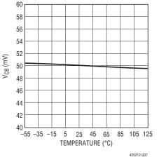
Undervoltage Lockout V<sub>LKO</sub> vs Temperature
