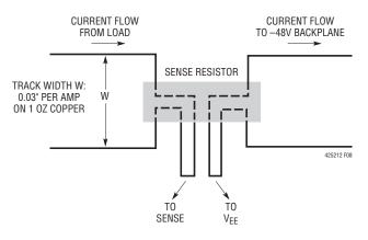
Figure 8. Making PCB Connections to the Sense Resistor
