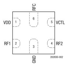
Figure 2. SKY13453-385LF Pinout (Top View)
