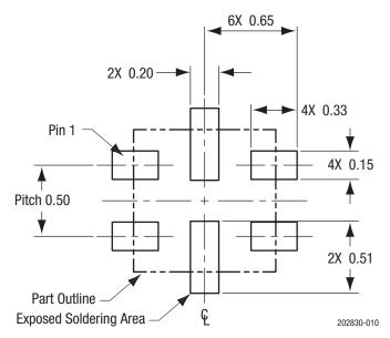
Figure 10. SKY13453-385LF PCB Layout Footprint (Top View)
