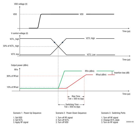
Figure 3. SKY13453-385LF Timing Diagram
