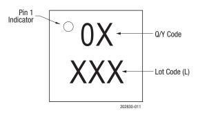
Figure 11. Typical Part Markings (Top View)
