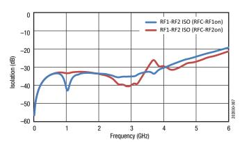
**Figure 6. Isolation vs Frequency**
