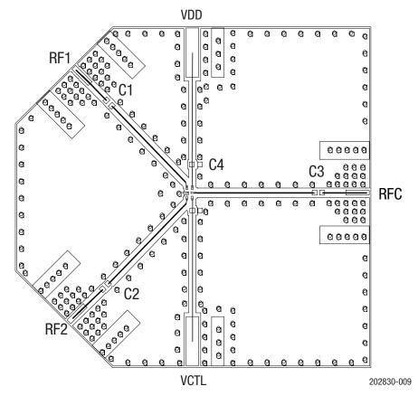
Figure 9. SKY13453-385LF Evaluation Board Assembly Diagram
