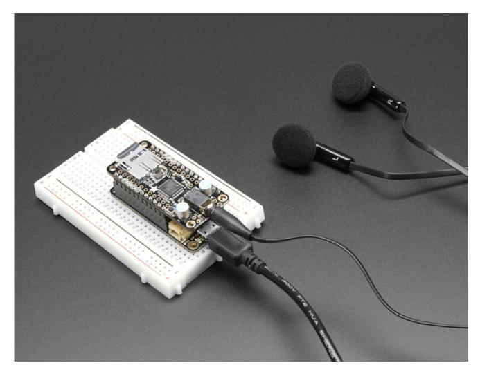
Bend all audio files to your will with the Adafruit Music Maker Feather Wing! It's a fun-size version of our Music Maker shield for Arduino (http://adafru.it/tbM)! This powerful shield features the VS1053, an encoding/decoding (codec) chip that can decode a wide variety of audio formats such as MP3, AAC, Ogg Vorbis, WMA, MIDI, FLAC, WAV (PCM and ADPCM). You can do all sorts of stuff with the audio as well such as adjusting bass, treble, and volume digitally.
