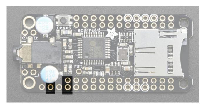
For powering the SD card and MP3 chip, we need power from the **3V** (2nd pin) and **GND** (4th pair of pins).
