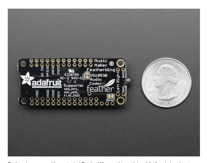
Each order comes with one tested FeatherWing, and two sticks of 0.1" male headers to plug it into your Feather and terminal blocks if you have the Amplifier version. Some light soldering is required to attach the through-hole headers to the PCB for plugging into your Feather Board. **Headphones**, **speakers**, **SD** card and Feather Board not included!
