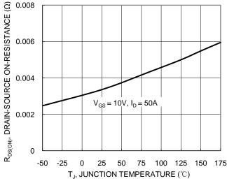
Figure 7. On-Resistance Variation with Temperature
