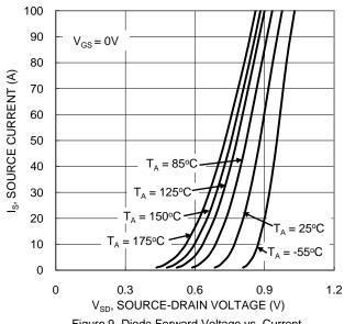
Figure 9. Diode Forward Voltage vs. Current
