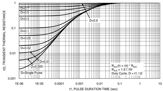
Figure 13. Transient Thermal Resistance
