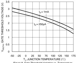
Figure 8. Gate Threshold Variation vs. Temperature
