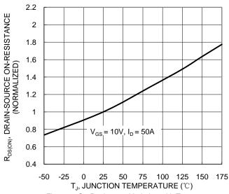
Figure 6. On-Resistance Variation with Temperature
