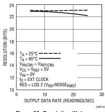
Figure 33. Resolution (Noise<sub>RMS</sub> ≤ 1LSB) vs Output Data Rate and Temperature
