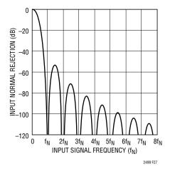
Figure 27. Input Normal Mode Rejection 2x Speed Mode
