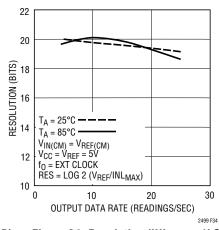
Figure 34. Resolution (INL<sub>MAX</sub>  $\leq$  1LSB) vs Output Data Rate and Temperature
