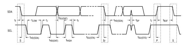
Figure 2. Definition of Timing for Fast/Standard Mode Devices on the I<sup>2</sup>C Bus
