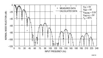
Figure 22. Input Normal Mode Rejection vs Input Frequency with Input Perturbation of 100% (60Hz Notch)
