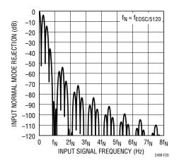
Figure 20. Input Normal Mode Rejection at DC
