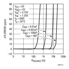
Figure 13. +FS Error vs R<sub>SOURCE</sub> at V<sub>REF</sub> (Small C<sub>REF</sub>)
