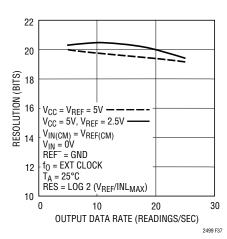
Figure 37. Resolution (INL<sub>MAX</sub> ≤ 1LSB) vs Output Data Rate and Reference Voltage
