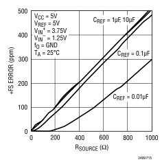
Figure 15. +FS Error vs R<sub>SOURCE</sub> at V<sub>REF</sub> (Large C<sub>REF</sub>)
