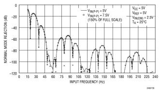
Figure 25. Measure Input Normal Mode Rejection vs Input Frequency with Input Perturbation of 150% (60Hz Notch)
