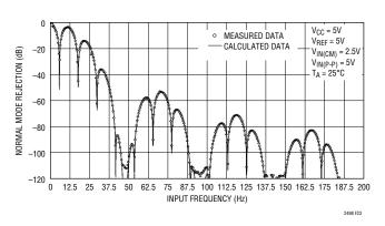
Figure 23. Input Normal Mode Rejection vs Input Frequency with Input Perturbation of 100% (50Hz Notch)
