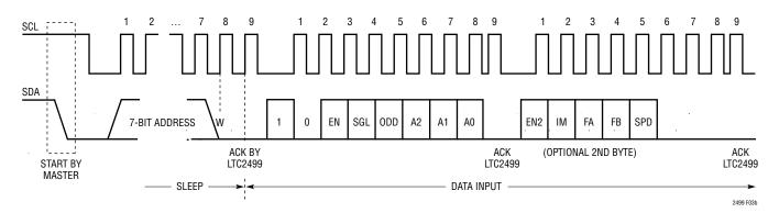
Figure 3b. Timing Diagram for Writing to the LTC2499
