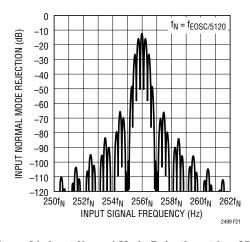
Figure 21. Input Normal Mode Rejection at  $f_S = 256 \bullet f_N$
