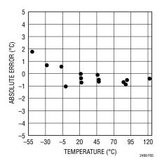
Figure 5. Absolute Temperature Error
