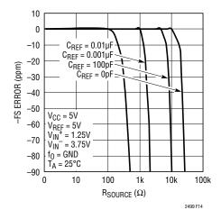
Figure 14. -FS Error vs R<sub>SOURCE</sub> at V<sub>REF</sub> (Small C<sub>REF</sub>)
