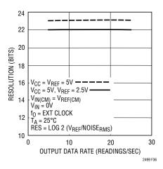
Figure 36. Resolution (Noise<sub>RMS</sub> ≤ 1LSB) vs Output Data Rate and Reference Voltage
