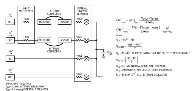
Figure 11. Equivalent Analog Input Circuit
