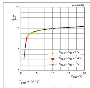
Fig. 3. Output current as a function of supply voltage; typical values
