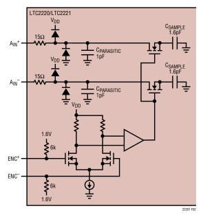
Figure 2. Equivalent Input Circuit
