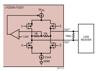
Figure 13b. Digital Output in LVDS Mode
