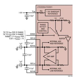
Figure 9. Equivalent Reference Circuit
