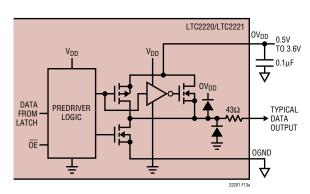
Figure 13a. Digital Output Buffer in CMOS Mode
