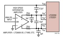
Figure 4. Differential Drive with an Amplifier
