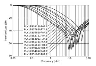
Common Mode Insertion Loss-Frequency Characteristics
