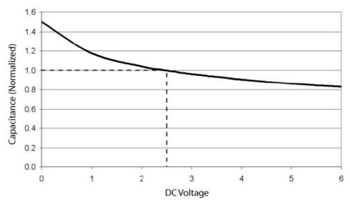
Figure 13. Filter Capacitance vs. Input Voltage over Temperature (normalized to capacitance at 2.5 V DC and 25°C)
