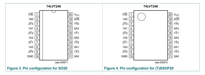
3.3 V Octal inverting buffer/line driver; 3-state
