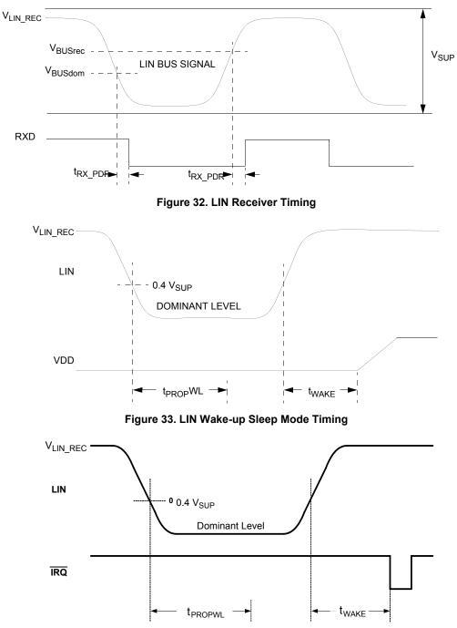
Figure 34. LIN Wake-up Stop Mode Timing
