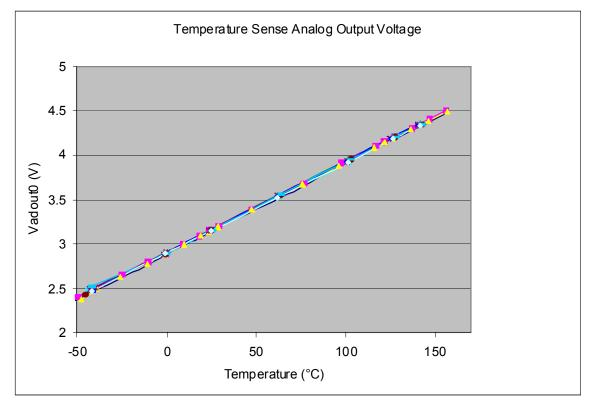
Figure 16. Temperature Sense Gain
