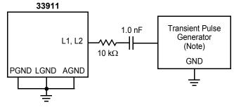
Note Waveform per ISO 7637-2. Test Pulses 1, 2, 3a, 3b,.
