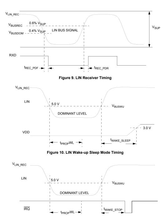
Figure 11. LIN Wake-up Stop Mode Timing
