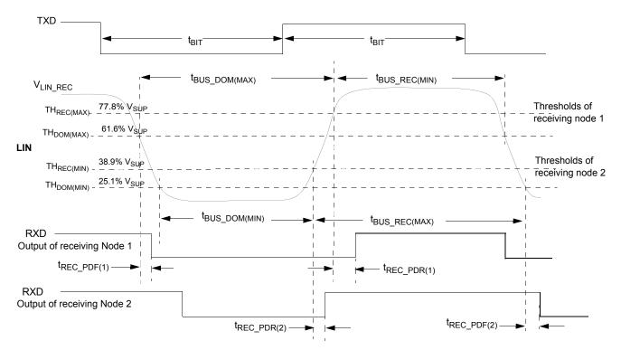
Figure 8. LIN Timing Measurements for Slow Slew Rate
