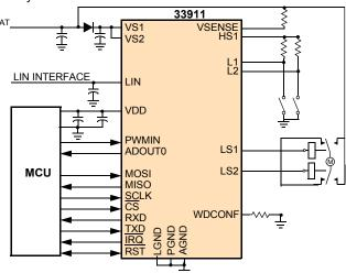
Figure 1. 33911 Simplified Application Diagram
