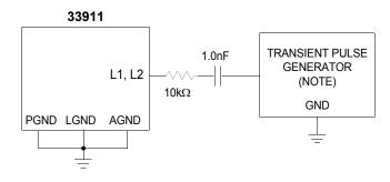
NOTE: Waveform per ISO 7637-2. Test Pulses 1, 2, 3a, 3b.
