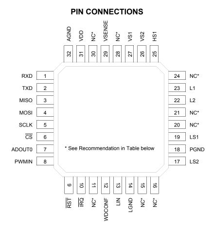
Figure 3. 33911 Pin Connections
