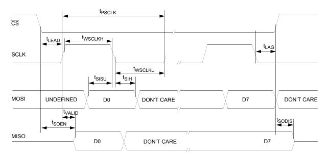
Figure 36. SPI Timing Characteristics
