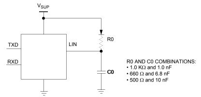
Figure 6. Test Circuit for LIN Timing Measurements
