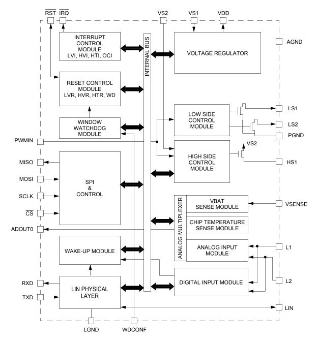
Figure 25. 33911BAC Simplified Internal Block Diagram
