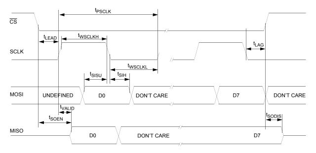
Figure 13. SPI Timing Characteristics
