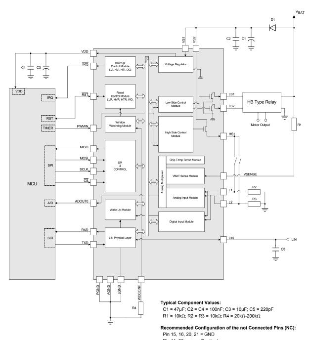
Pin 11, 30 = open (floating) Pin 24 = open (floating) or VS2 Pin 28 = this pin is not internally connected and may be used for PCB routing optimization.
