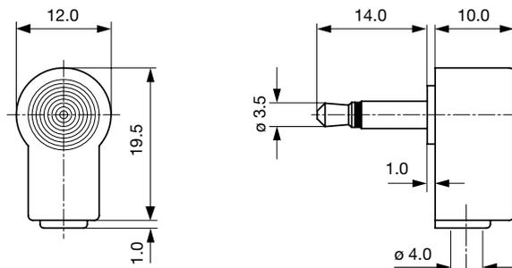
Cable diameter max. 4.0 mm
