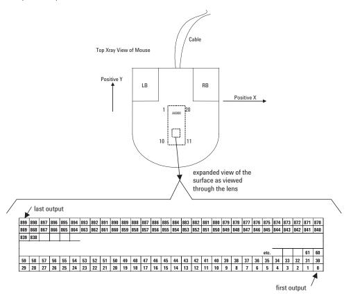
Figure 26. Pixel address map (surface referenced)
