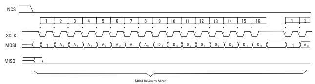
Figure 17. Write Operation
