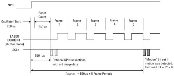
Figure 11. NPD Rising Edge Timing Detail
