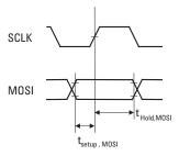
Figure 16. MOSI Setup and Hold Time
