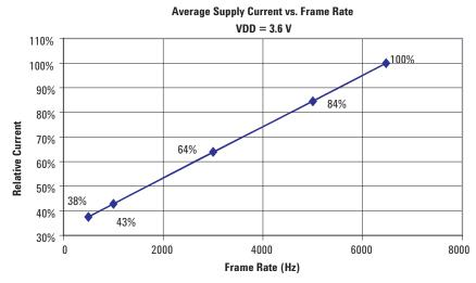
Figure 14. Average Supply Current vs. Frame Rate
