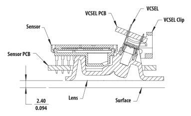
Figure 10. Distance from lens reference plane to surface
