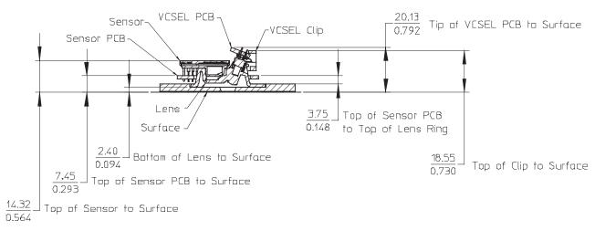
Figure 3. Assembly drawing of ADNS-6000 (top, front and cross-sectional view)
