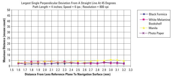
Relationship of mouse count to distance = m (mouse count) / n (cpi) eg: Deviation of 7 mouse count = 7/800 = 0.00875 inch  $\sim 0.009$  inch; where m = 7, n = 800 Figure 13. Average Error vs. Distance at 800cpi (mm)
