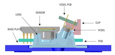
Figure 6. Cross section of PCB assembly
