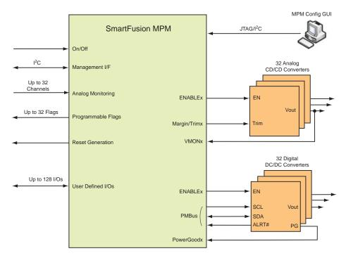
Microsemi's Mixed Signal Power Manager (MPM) reference design version 4.0 further distances itself from the competition by now including support for PMBus based POL converters. No other power management solution seamlessly supports a mix of analog and PMBus based power converters. Now you can sequence, monitor, and manage a mixed set of DC/DC converters, including LDOs, analog style, and the highly efficient PMBus based converters, from a single management device.
