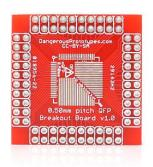
xQFP breakout board - 0.5mm
