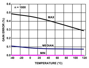
FIGURE 44. ISL28273 % GAIN ERROR vs TEMPERATURE,  $R_1 = 100k$
