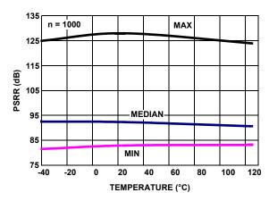
FIGURE 42. PSRR vs TEMPERATURE, V<sub>+</sub>, V<sub>-</sub> = ±1.2V TO ±2.5V
