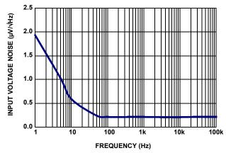
FIGURE 16. ISL28273 INPUT VOLTAGE NOISE SPECTRAL DENSITY (GAIN = 10)
