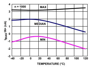
FIGURE 29. IBIAS IN+ vs TEMPERATURE, V+, V- = ±1.2V
