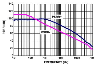
FIGURE 13. ISL28270, ISL28470 PSRR vs FREQUENCY
