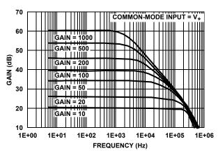
FIGURE 2. ISL28273 FREQUENCY RESPONSE vs CLOSED LOOP GAIN,  $V_{CM} = V_{+} = 5V$
