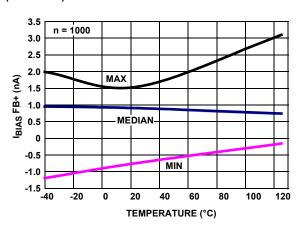
FIGURE 30. I<sub>BIAS</sub> FB+ vs TEMPERATURE, V<sub>+</sub>, V<sub>-</sub> = ±1.2V
