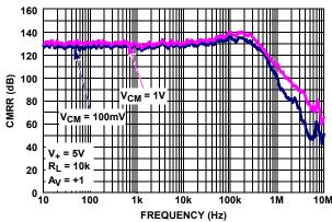
FIGURE 12. ISL28273 CMRR vs FREQUENCY
