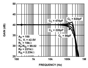
FIGURE 9. ISL28270, ISL28470 FREQUENCY RESPONSE vs C<sub>LOAD</sub>
