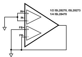
FIGURE 52. PREVENTING OSCILLATIONS IN UNUSED CHANNELS
