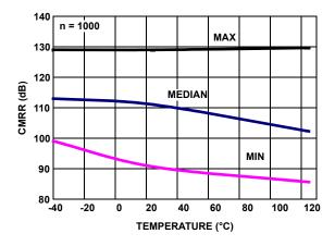
FIGURE 41. CMRR vs TEMPERATURE, VCM = +2.5V TO -2.5V,  $V_+$ ,  $V_-$  = ±2.5V
