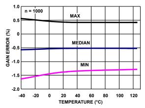
FIGURE 43. ISL28270, ISL28470 % GAIN ERROR vs TEMPERATURE,  $R_{\rm L}$  = 100k
