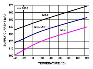
FIGURE 23. SUPPLY CURRENT (CHANNEL A AND CHANNEL B) vs TEMPERATURE,  $V_+, V_- = \pm 2.5 V, V_{\mbox{\scriptsize IN}} = 0 V,$   $R_L = \mbox{\scriptsize INF}$
