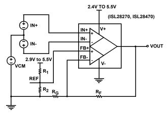
FIGURE 50. GAIN SETTING AND REFERENCE CONNECTION
