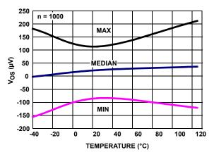
FIGURE 37. ISL28270, ISL28470  $V_{OS}$  vs TEMPERATURE,  $V_+, V_-$  = ±2.5V
