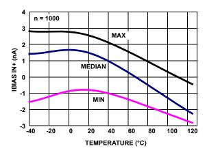
FIGURE 25. IBIAS IN+ vs TEMPERATURE, V+, V = ±2.5V
