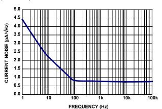
FIGURE 18. ISL28273 INPUT CURRENT NOISE SPECTRAL DENSITY (GAIN = 10)
