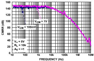
FIGURE 11. ISL28270, ISL28470 CMRR vs FREQUENCY
