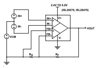
FIGURE 49. GAIN IS SET BY TWO EXTERNAL RESISTORS,  $\rm R_F$  AND  $\rm R_G$
