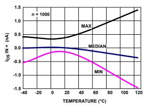
FIGURE 35. IOS IN+ vs TEMPERATURE, V<sub>+</sub>, V<sub>-</sub> = ±1.2V
