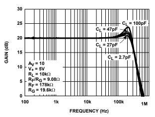
FIGURE 10. ISL28273 FREQUENCY RESPONSE vs CLOAD
