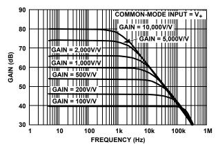
FIGURE 1. ISL28270, ISL28470 FREQUENCY RESPONSE vs CLOSED LOOP GAIN,  $V_{CM} = V_{+} = 5V$
