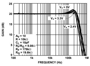
FIGURE 8. ISL28273 FREQUENCY RESPONSE vs SUPPLY VOLTAGE
