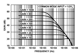
FIGURE 4. ISL28273 FREQUENCY RESPONSE vs CLOSED LOOP GAIN. V<sub>+</sub> = 5V, V<sub>CM</sub> = 1/2V<sub>+</sub>
