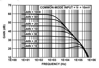
FIGURE 6. ISL28273 FREQUENCY RESPONSE vs CLOSED LOOP GAIN,  $V_+ = 5V$ ,  $V_{CM} = 10 \text{mV}$
