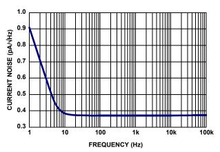
FIGURE 17. ISL28270, ISL28470 INPUT CURRENT NOISE SPECTRAL DENSITY (GAIN = 100)
