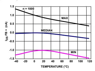
FIGURE 36. IOS FB+ vs TEMPERATURE, V<sub>+</sub>, V<sub>-</sub> = ±1.2V
