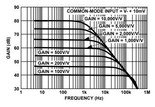
FIGURE 5. ISL28270, ISL28470 FREQUENCY RESPONSE vs CLOSED LOOP GAIN,  $V_+ = 5V$ ,  $V_{CM} = 10 \text{mV}$
