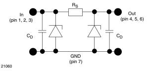
Each filter is symmetrical so that both ports can be used as input or output.
