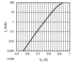
Fig. 3 - Typical Forward Current I<sub>F</sub> vs. Forward Voltage  $V_F$
