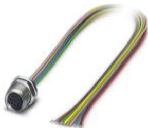
Sensor/actuator flush-type socket, 8-pos., M8, rear/screw mounting with M10 fastening thread, with 0.5 m TPE litz wire, 8 x 0.14 mm 2
