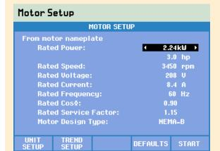
Input details of the motor from the rating plate including rated power, rated speed and motor type from either NEMA or IEC classifications.
