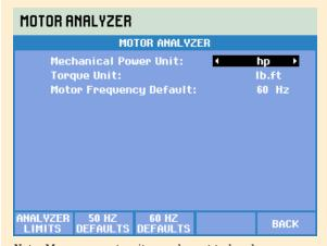
Note: Measurement units can be set to local requirements hp/kW, lb ft/Nm etc.
