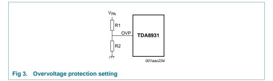
The overvoltage protection level can be determined by the formula:
