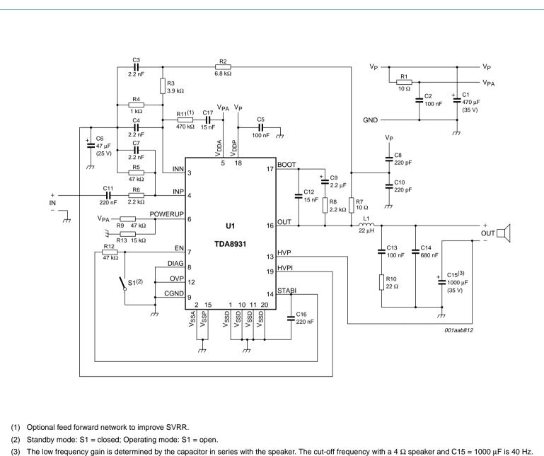
Fig 5. Typical application diagram with TDA8931 supplied from an asymmetrical supply
