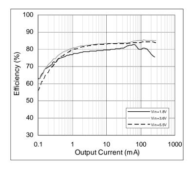
Figure 8: Efficiency vs. Output Current; V<sub>OUT</sub> = 3.0V
