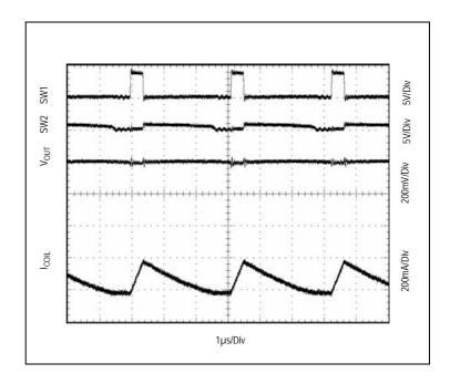
Figure 26: Startup;  $V_{IN}$  = 3.6V,  $R_{load}$  = 3.3k $\Omega$
