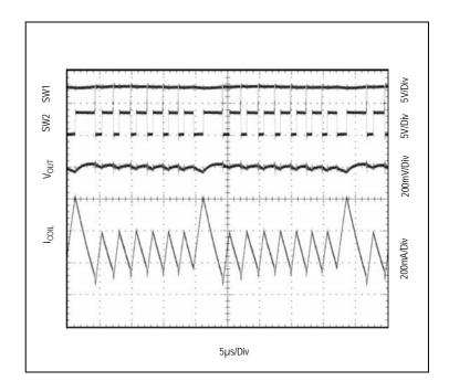
Figure 24:  $V_{IN} = 2.5V$ ,  $V_{OUT} = 3.3V$ ,  $I_{OUT} = 50$ mA
