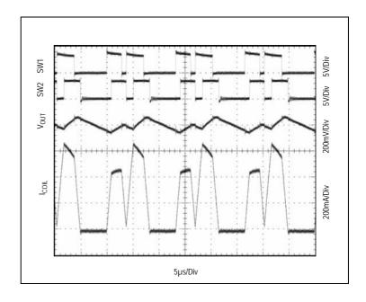
Figure 22:  $V_{IN} = 3.6V$ ,  $V_{OUT} = 3.3V$ ,  $I_{OUT} = 50$ mA
