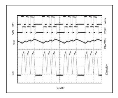
Figure 20:  $V_{IN} = 4.4V$ ,  $V_{OUT} = 3.3V$ ,  $I_{OUT} = 50$ mA
