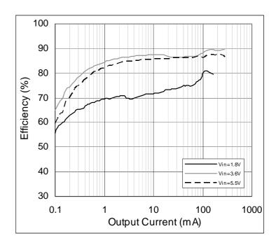
Figure 10: Efficiency vs. Input Voltage
