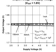
Output Voltage vs Supply Voltage
