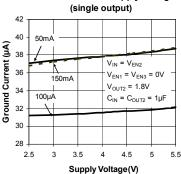
Ground Current vs Supply Voltage
