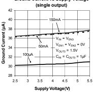
Ground Current vs Supply Voltage
