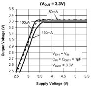
Output Voltage vs Supply Voltage
