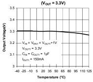
Output Voltage vs Temperature
