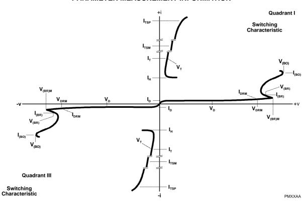
Figure 1. VOLTAGE-CURRENT CHARACTERISTIC FOR ANY PAIR OF TERMINALS
