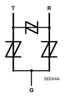
Terminals T, R and G correspond to the alternative line designators of A, B and C
