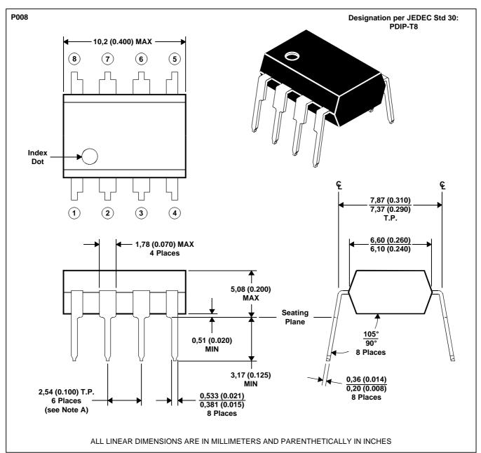
NOTE A: Each pin centerline is located within 0,25 (0.010) of its true longitudinal position
