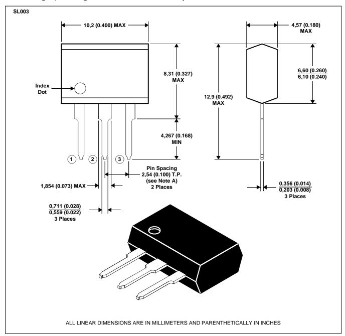
NOTES: A. Each pin centerline is located within 0,25 (0.010) of its true longitudinal position.
