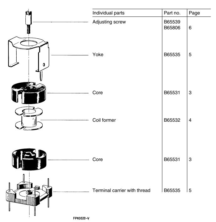
Example of an assembly set for printed circuit boards
