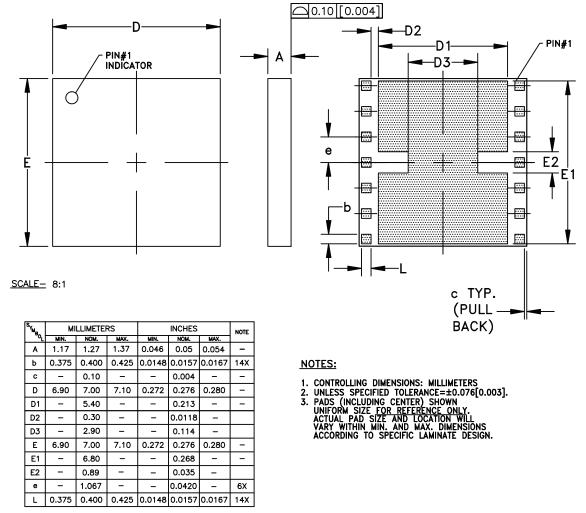
Figure 5: Package Outline - 14 Pin 7 mm x 7 mm x 1.3 mm Surface Mount Module
