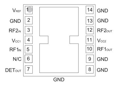
Figure 2: Pinout (X-ray Top View)
